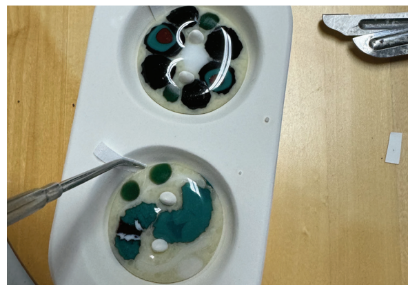
ThinFire tab assists removal
